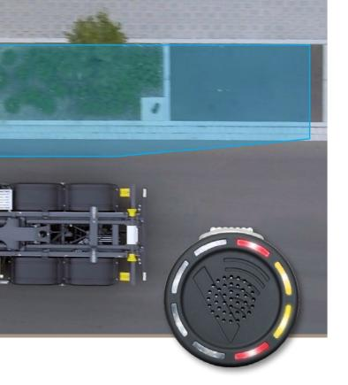
The LED display on the A-pillar provides the driver with visual alerts. When the turn signal is activated, an additional audible alert is generated.
