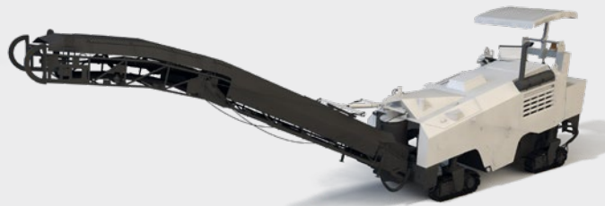
Road Milling Machine
