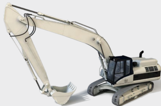
Long Front Excavator
