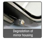
The test results greatly deviate from MEKRA Lang standards and would clearly be disqualifiers for our own mirrors. Using products with such quality deficiencies on the road and in freight traffic could result in significant safety risks.
